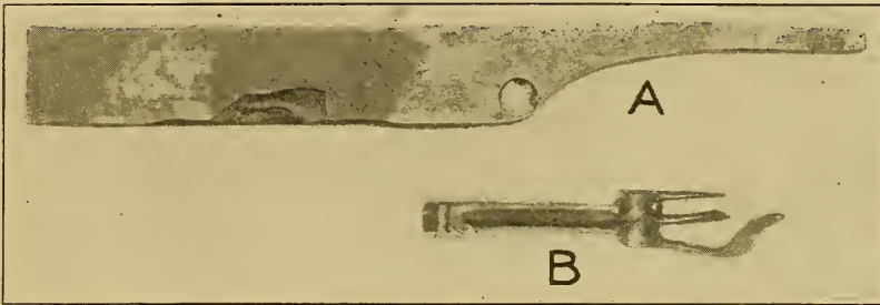
Fig. 137. Worn Parts of Loom Causing Failure to Stop.
